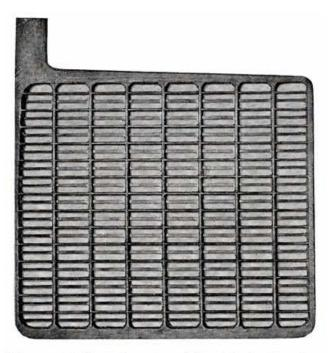
Fig. 4. Grid, Trimmed, and Ready for Pasting
