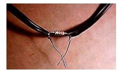
When fast charging is needed the resistor leads are connected together and the resistor is effectively taken out of the circuit. In the above example we used a 220 ohm resistor. One way to find the right value of resistance is to temporally hook up a digital amp meter and a variable resistor (pot) and adjust the flow to be about 100 times less current than what is measured when the pot is zero ohms. Then measure the resulting resistance using a digital ohm meter.
