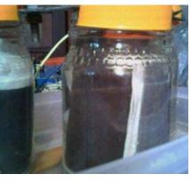
2 was weak, so I replaced the plate with a fresh sheet of lead. While busy, I couldn't resist jabbing holes in both sides of the plates with a clean compass point, and also scratching crossed diagonal lines into both sides. Hopefully this will increase the initial surface area, and allow the sponge-forming to penetrate more deeply.
