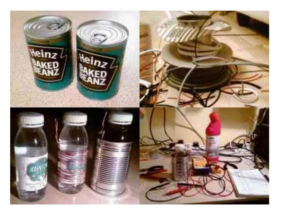
Above, the construction process. One cell uses one baked bean can. I liked baked beans, and anyway I have a collection of baked bean cans because they are great as shielding material, or as circuit substrate for "ugly" construction. Next comes the "other" electrode, for which I used copper wire again. The copper wire is from a bit of old house lighting cable, left over on a reel. I have grey and
