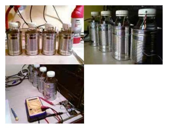
I built FOUR of these baked bean can cells, and connected them in series. One 750ml bottle of ASDA thick bleach costs 60 or 70 pence and is more than enough to fill all four cells and clean the toilet too. The voltage of the four cells is more than 3V. I connected the homebrew battery up to my <u>40m QRSS transmitter</u> - it's the circuit in the bottom right corner of the photo, 3'rd from left. That circuit is built on a baked bean can tin substrate too!
